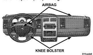
This vehicle has airbags for both the driver and right front passenger as a supplement to the seat belt restraint systems. The driver's front airbag is mounted in the steering wheel. The passenger front airbag is mounted in the instrument panel, above the glove compartment. The words SRS/AIRBAG are embossed on the airbag covers.
